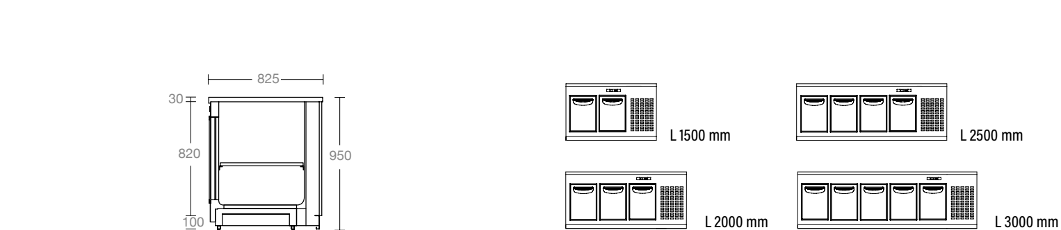
BANCO CON CELLE REFRIGERATE STATICHE E MOTORE INCORPORATO H950 P825 MM COUNTER WITH STATIC REFRIGERATED ROOMS & HERMETIC UNIT H950 D825 MM
